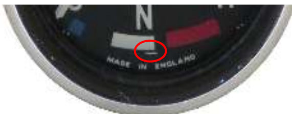
Figure 29: Gauge scale showing mid-point calibration "bar" in lieu of the more usual dots.
