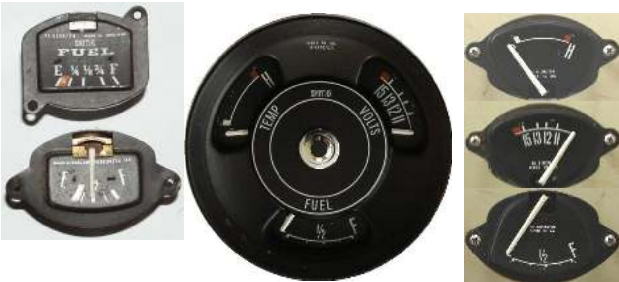
Figure 2: Photos showing the two styles of “quadrant” gauge on the left and an instrument panel and its associated gauges on the right. Panel from a Triumph 2000 Mk II
