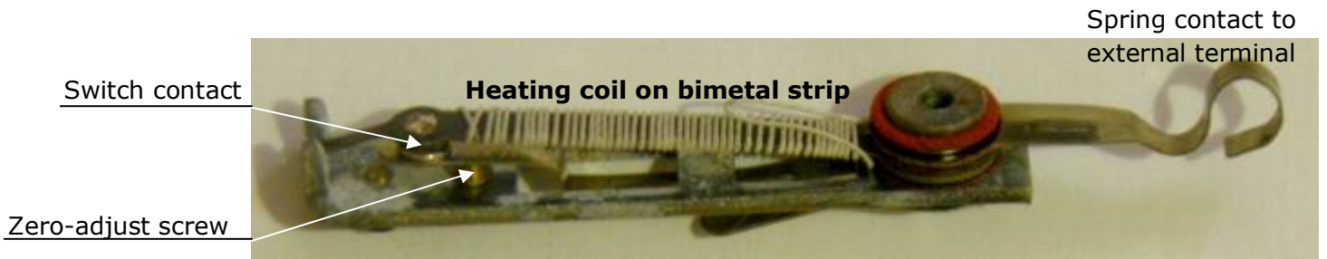
Figure 7: Bimetal temperature sensing element (Aftermarket unit but similar to Smiths sender.)
