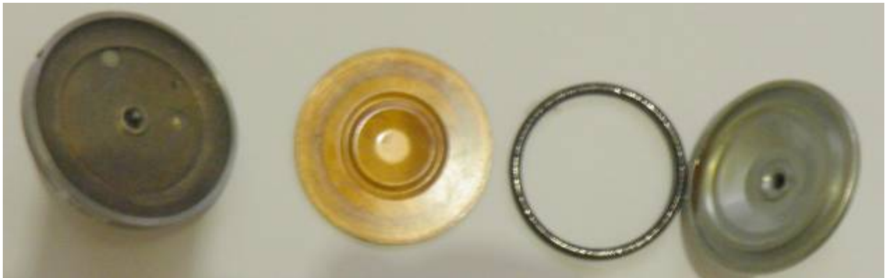
Figure. 22: Lower portion of bimetal pressure transmitter .
