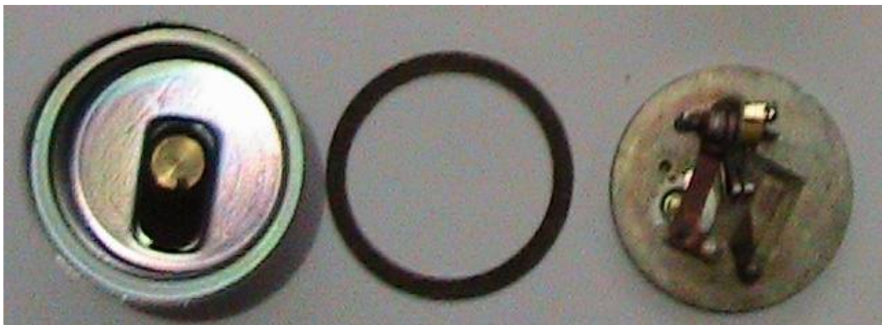
Figure. 23: Sender mechanism of bimetal pressure sender .
