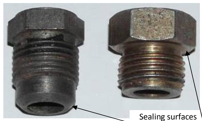
Figure 15: The difference between a TT380x and TT480x is in the collar – TT380x (bevel or cone seal) on left , TT480x (face seal) on right.
